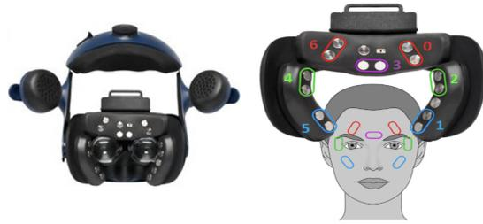
**Figure 1:** emteqPRO™ multi-sensor face mask.
